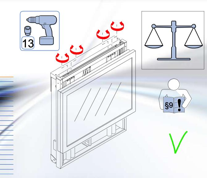
Balance the weight on the BalanceBox® 650 by loosening (rotate counter clockwise) the 4 outermost bolts.
